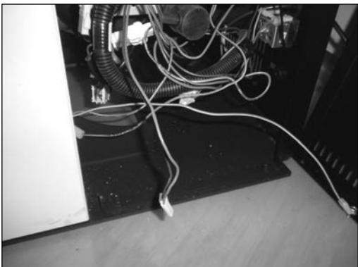
The two blade receptacles are of different sizes and therefore cannot be connected to the cross-flow fan incorrectly.
