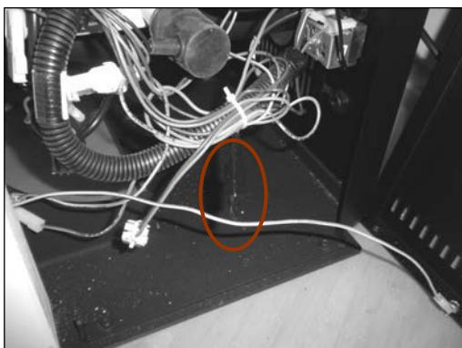
Remove the heat-shrink tubing and the insulating sheath of the cross-flow fan connections (blue and brown cable).
