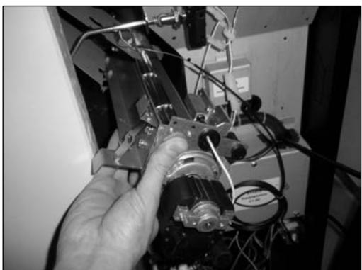
Insert the cross-flow fan into the stove from the right-hand side.
