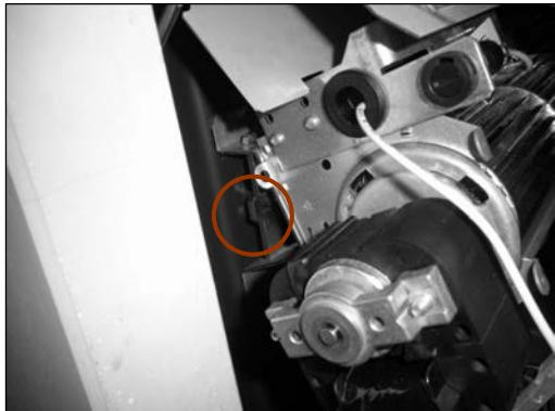
The cross-flow fan can now be mounted on the set screws.
