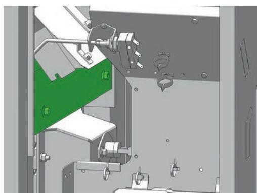
Remove the two nuts from the heat protection sheet. Remove the heat protection sheet, it is not used anymore.
