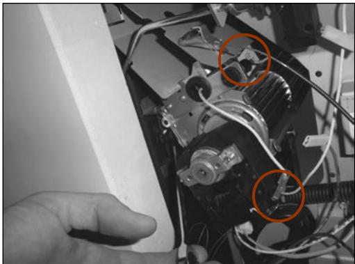
Secure the cross-flow fan in place using the two supplied washers and hexagonal nuts. Connect the two blade receptacles (cable harness) to the two blade terminals (fuse and motor) on the cross-flow fan.
