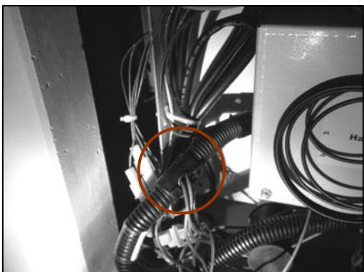
Open the connecting piece (cable outlet) on the cable harness and pull the two cross-flow fan cables from the protective tube. Close the connecting piece (cable outlet) again.
