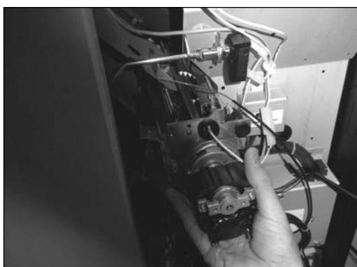
When it has been inserted halfway turn the cross-flow fan gently counter-clockwise and position it level with the set screws that are intended for its attachment.
