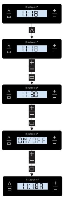
By pressing the  $\mbox{ON}$  /  $\mbox{OFF}$  button the programed ignition time can be activated or deactivated.
