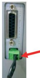
Remove the cable bridge from the stove's interface and connect the cable of the room thermostat in its place.
