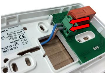
Now connect the 2-pin cable to positions 1 and 2 of the terminal block.
