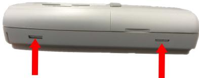
Use a suitable tool to depress the opening button and remove the cover from your room thermostat.
