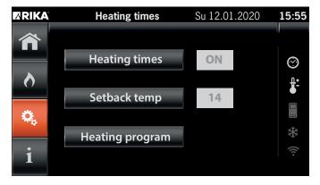
In the heating times program, single weekdays, or a couple of weekdays can be marked simultaneously (highlighted in ORANGE).
