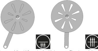
In general the riddle grate should stay open. The air regulation is made completely with the control knob at the rear wall.
