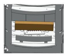
Start stove operation. After ignition has been successful, the operating state **IGNITION** switches to **LOG CHECK**, and after successful log recognition to **LOG OPERATION**.
