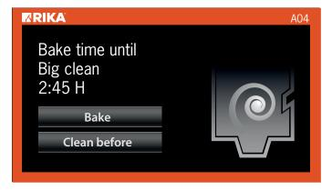
Select **BAKE** if the remaining time displayed is sufficient for your baking operation.
