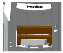
Now place more chipboard pieces crossways and add 2-4 ribs of the RIKA firelighter on top of the chipboard. If necessary, some uncoated paper can be placed under the chipboard instead of the firelighter.
