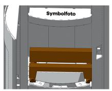
2. Now place further pieces of chipboard in crosswise layers on top of the logs and place 2-4 ribs of the RIKA-firelighter on the left on top of the chipboard. Some uncoated paper can be placed underneath the chipboard in case there is no firelighter available.
