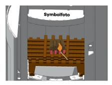
3. Now light the firelighter (or the uncoated paper) and close the combustion chamber door. "Correct heating up" primarily counteracts excessive smoke during heating up.
